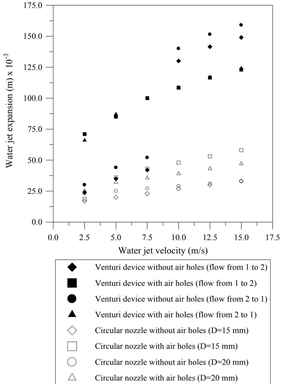
**Fig. 4.** Variation in Water Jet Expansion with Water Jet Velocity for Venturi and Circular Nozzles
