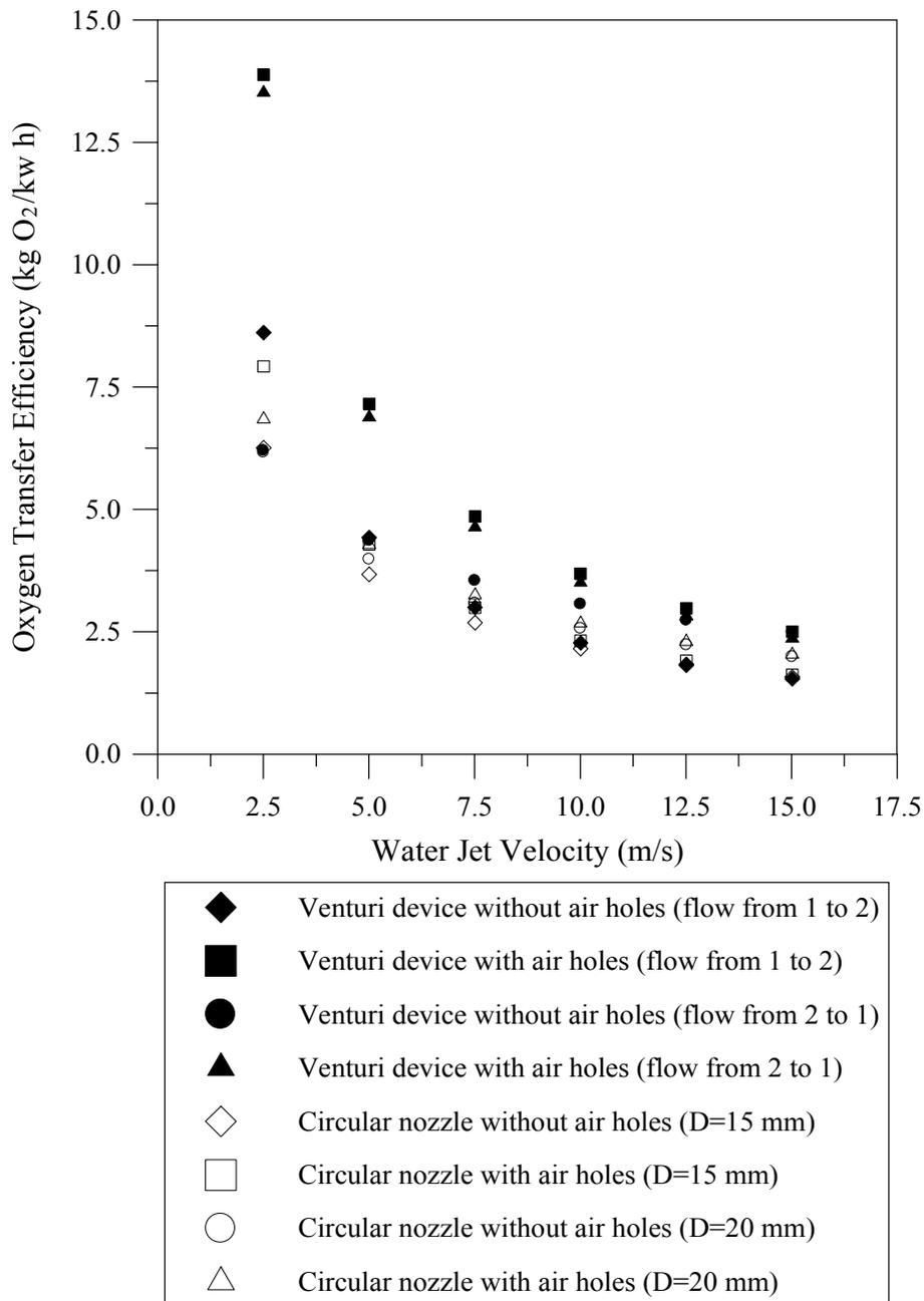
Fig. 6. Variation in Oxygen Transfer Efficiency with Water Jet Velocity for Venturi and Circular Nozzles
