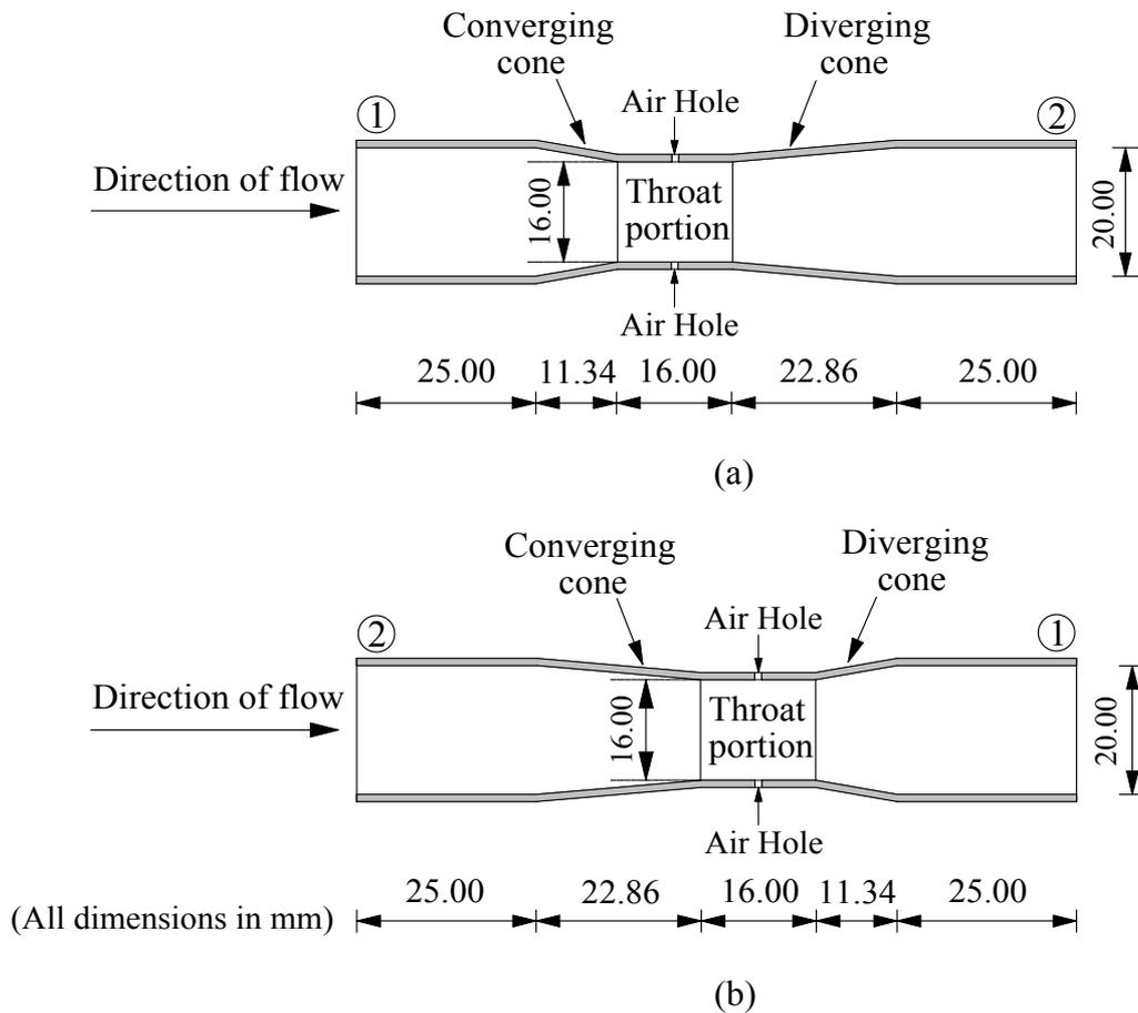
Fig. 1. Details of Venturi Nozzle (a) Direction of Flow from 1 to 2; (b) Direction of Flow from 2 to 1
