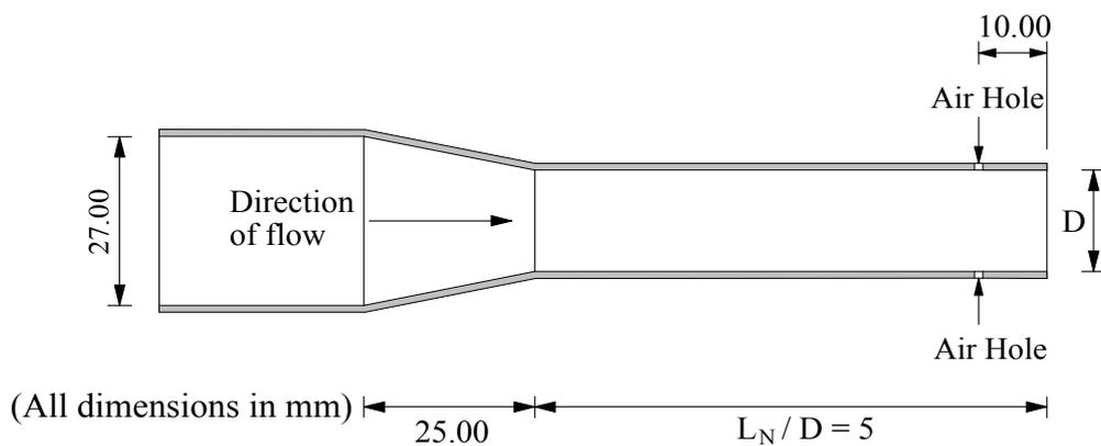
Fig. 2. Details of Circular Nozzle with Air Holes
