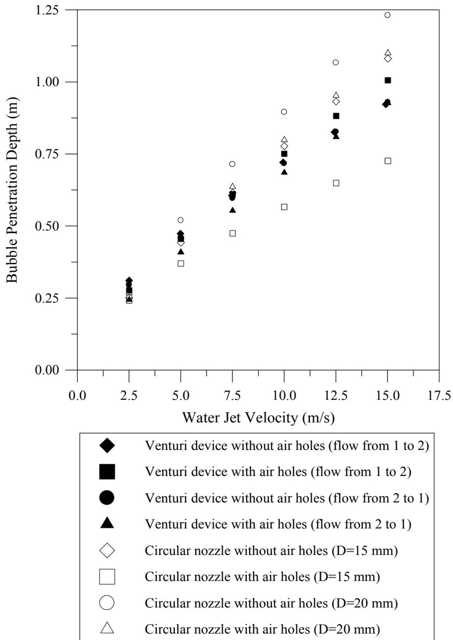
**Fig. 5.** Variation in Bubble Penetration Depth with Water Jet Velocity for Venturi and Circular Nozzles
