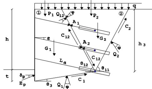
Figure 4: Kinematical model by the failure of the lower anchor.
